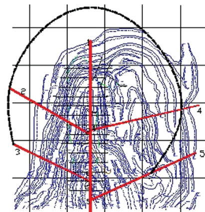
Fig. 10. Zone of the rock displacement in the north part of the Ushkatyn-3 mine
